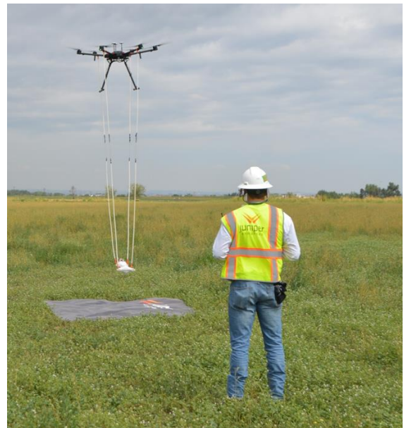
Drone Based Magnetometer System Mapping Abandoned Oil Wells and Flow Lines in Colorado
